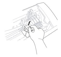
Open the new ink cartridge bag for the colour on the display and remove the ink cartridge. 8 Hold the ink cartridge as shown in the illustration, and remove the sealing tape from the side of the ink cartridge. Carefully peel the tape in the direction away from you..
